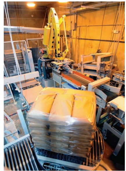
The packaging line’s stretch wrapper automatically wraps and secures a completed pallet for transport.
