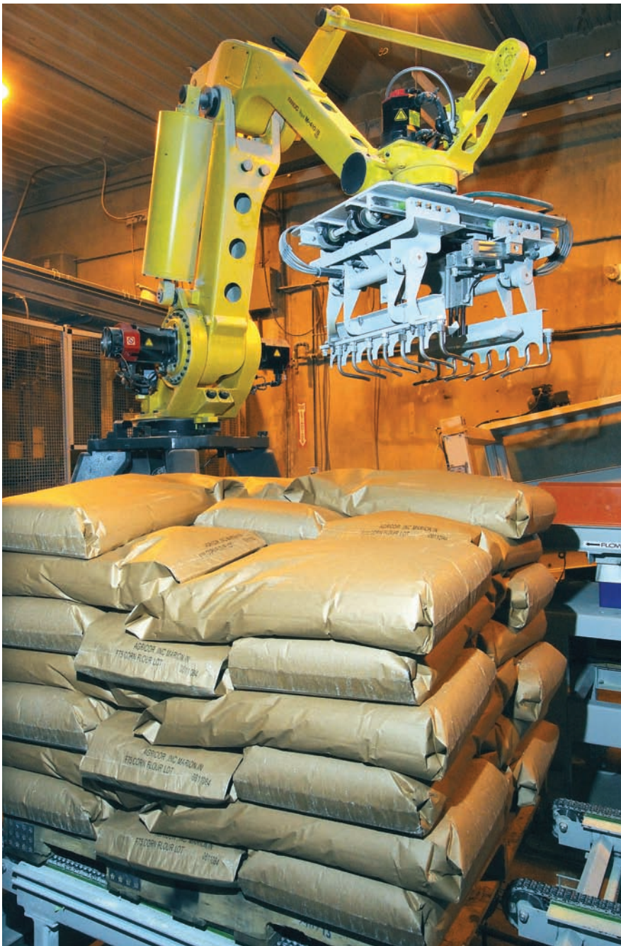
The robotic arm's finger gripper can easily handle multiple bag sizes, from 9 by 13 by 1.5 inches up to 23 by 39 by 6 inches.
