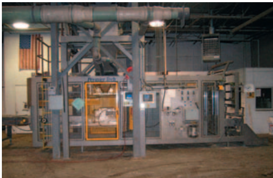
The FFS machine makes handled and handleless plastic bags, packaging both the ice-melting and construction products in various-sized plastic bags.
