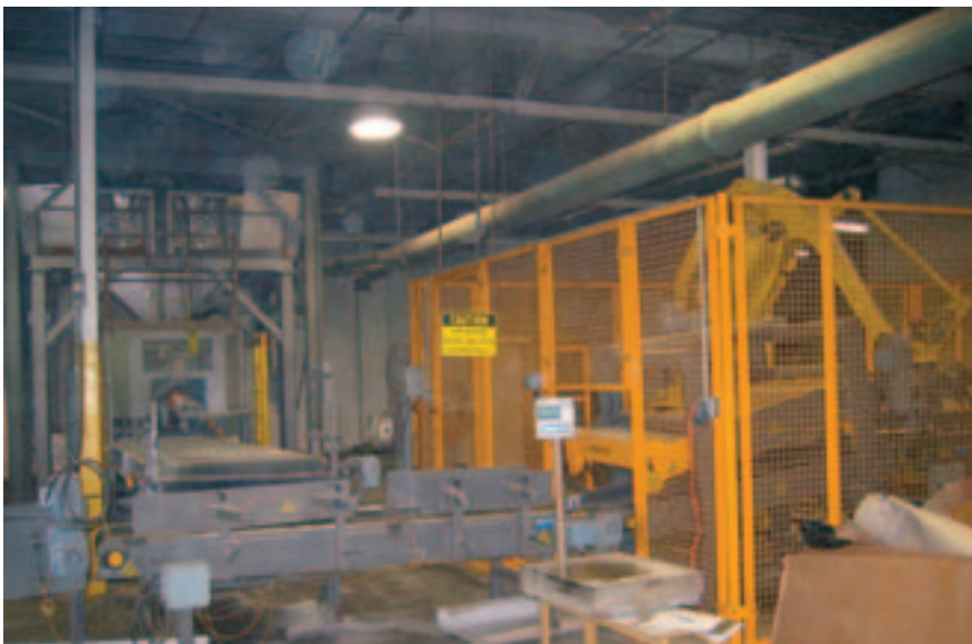
The robotic palletizer, which sits in the middle of the production area, receives plastic bags from the form-fill-seal machine and paper bags from the other bagging station.
