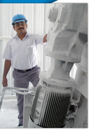
"We've achieved our goal of reducing energy and nitrogen consumption when conveying PTA by replacing the 320 kWh pneumatic conveyor with a 25-horsepower tubular drag conveyor."
