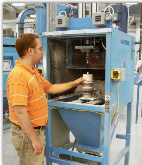
Knock out station with specially designed apparatus and integral dust hood reduces dust created during the plaster knock-out process, preventing equipment problems and improving the work environment.
