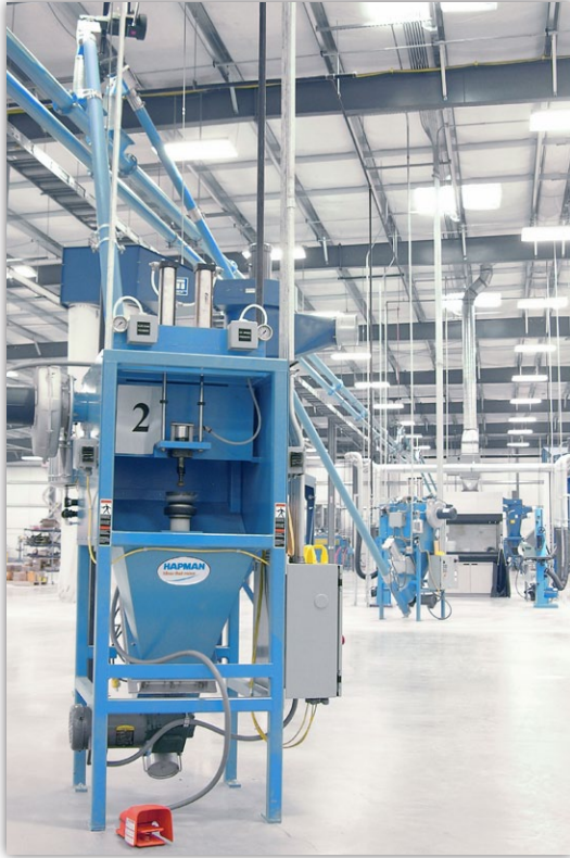
Custom knock-out station with attached Helix flexible screw conveyor that moves the lightweight, chunky plaster to the tubular drag conveyor for removal to an outside receptacle.
